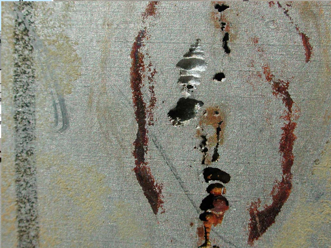
Figure 12. Nonuniform (patchy) colonization by bacteria in differential aeration cells. This schematic shows pit formation due to oxygen depletion under a biofilm. (Borenstein 1994)
