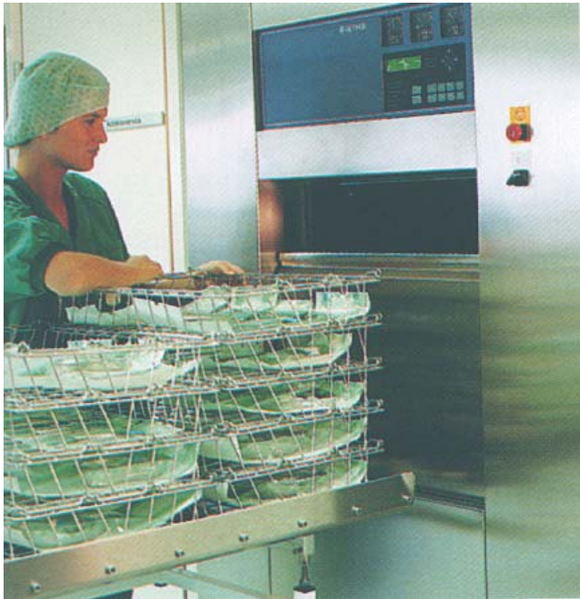
The Getinge 2066-series LTSF sterilizer, with chamber opening 672 x 672 mm.
