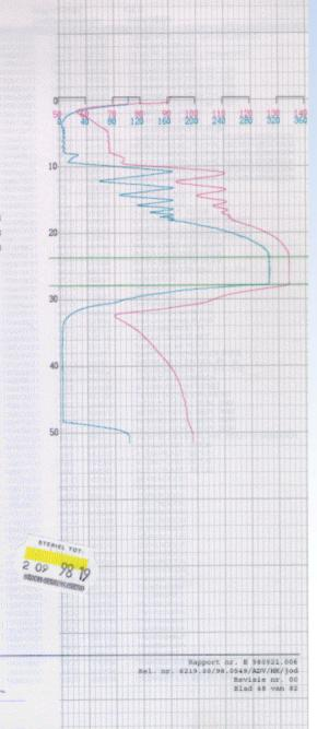
Print and diagram of a steam sterilization process used for parametric release
