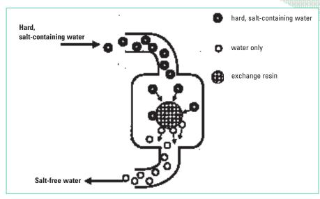
Fig. 2: Principle of complete demineralisation by ion exchange
