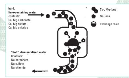
Fig. 1: Pinciple of water softening
