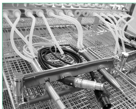
Fig. 3 – 5: Different loading trolleys with connections and adaptors for ophthalmologic instruments
